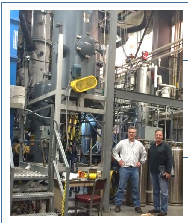
1 MWE CHP SKID MOUNTED FACTORY ASSEMBLED
